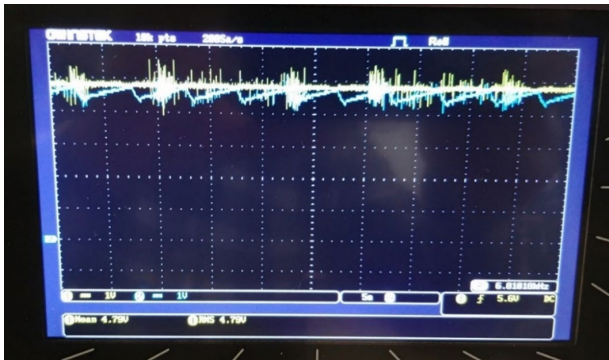
Fig. 11: Oscilloscope waveform of output and supercapacitor voltages at 1.75 watts.
